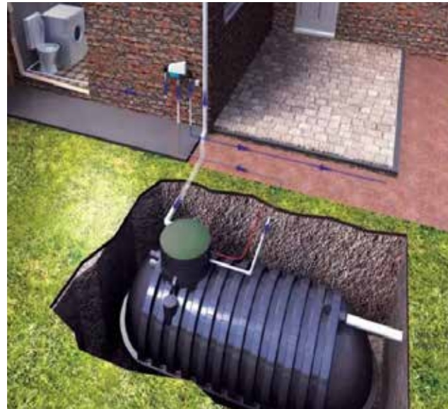
Figure 86: Example of an underground water tank in relationship with the building (Source: https://handymantips.org/about-underground-water-tanks/ )
