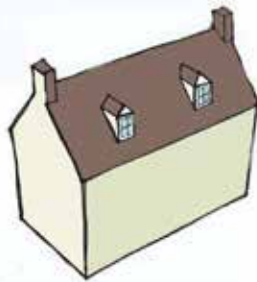
Loft conversion incorporating gabled dormers.
